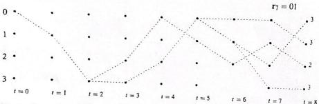
The decoding is finalized at the end of the transmission (the 16 received data bits) by selecting the state at the last stage having the lowest cost, traversing backward along the path so indicated to the beginning of the trellis, then traversing forward again along the best path, reading the input bits and decoded output bits along the path. This is shown with the solid line below; input/output pairs are indicated on each branch.
