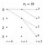
t=2: The received sequence is  $\mathbf{r}_2=00$ . Each path at time t=2 is extended, adding the path metric to each branch metric of each path.
