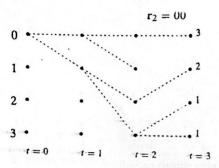
t = 3: The received sequence is  $r_3 = 10$ . Each path at time t = 3 is extended, adding the path metric to each branch metric of each path.
