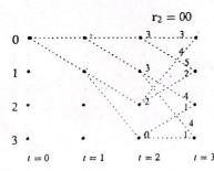
There are now multiple paths to each node at time t = 3. We select the path to each node with the best metric and eliminate the other paths. This gives the diagram as follows:
