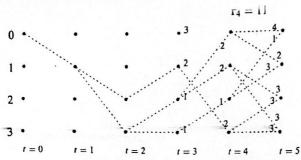
In this case, we note that there are multiple paths into state 3 which both have the same path metric; also there are multiple paths into state 2 with the same path metric. Since one of the paths must be selected, the choice can be made arbitrarily (e.g., at random). After selecting and pruning of orphan paths we obtain:
